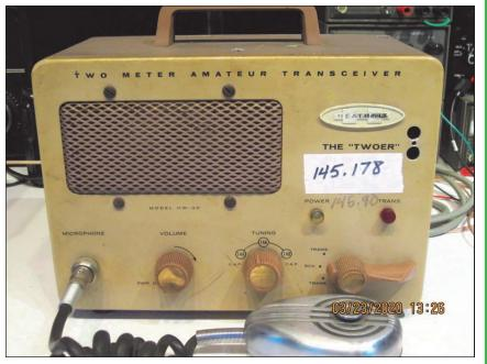
The Twoer has real plate modulation and with a good mike and careful adjustment of the final amp tuning it will make very nice AM transmit audio. The 750 mW carrier will modulate up to about a watt and a half on voice peaks. The transmitter uses 8 MHz crystals which were commonly available back in the day, multiplied 18 times to get to the 2 meter band.
